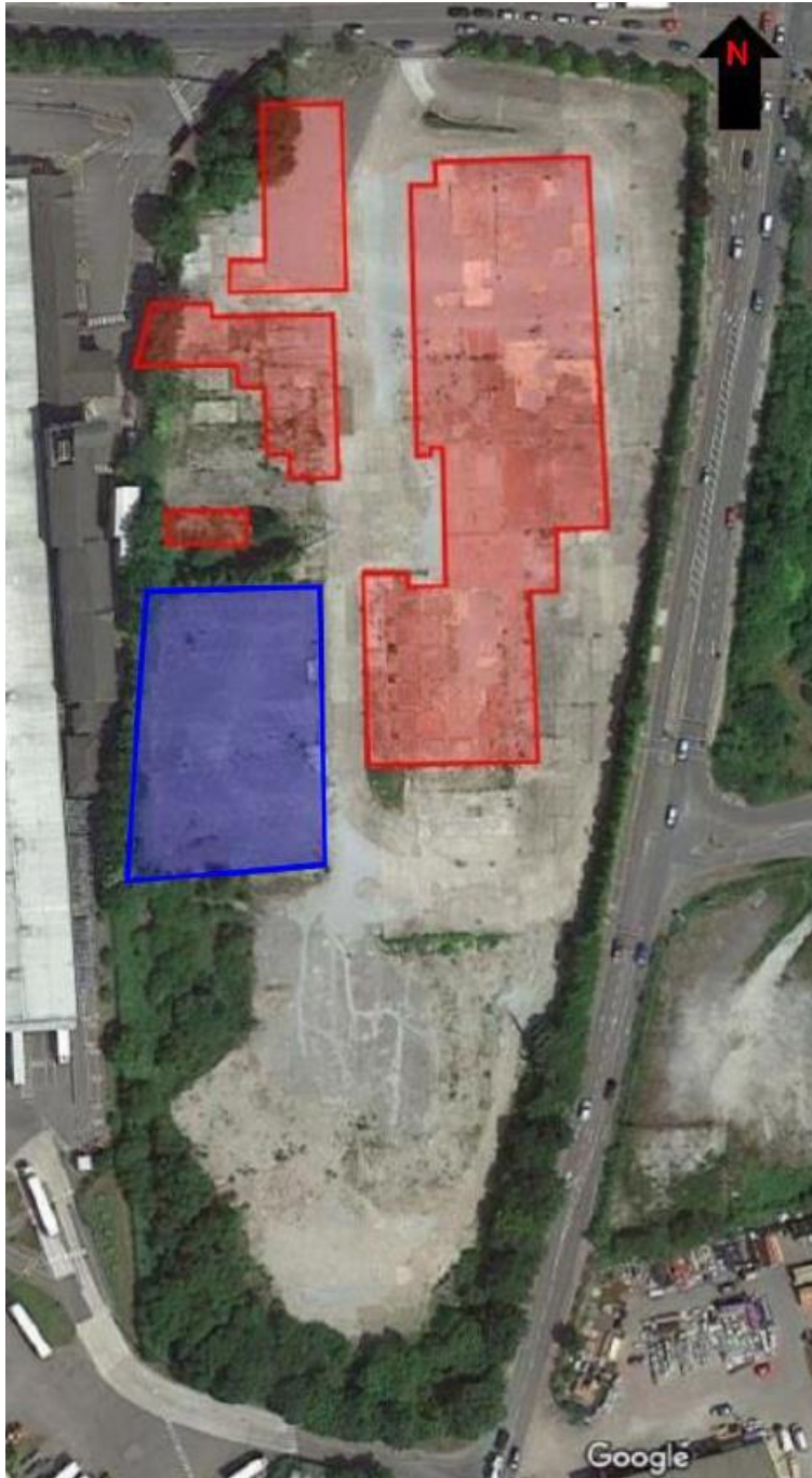
Figure 3: Extract from Google Maps marked up to show existing concrete ground slabs and foundations. Red: concrete floor slabs/foundations, blue: carpark.
